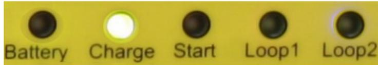
The LED marked 'Battery' indicates how much battery the ESD2 has left. Red light means the battery capacity is below 30%. Orange 30-60%. Yellow 60-90%. Green light means the battery capacity is over 90%. When fully charged the ESD2 has battery capacity for 10-12 hours use, depending on brightness and temperature.
