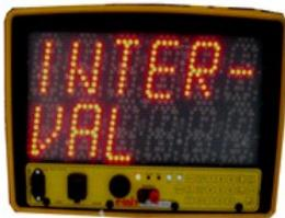
*Actual time (hh: mm: ss) is displayed on the top line, start number and countdown of seconds to next start is shown on the bottom line. The start time and the starting interval is entered manually by the keyboard.*
