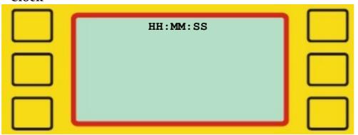
Use the numeric keys to set a valid time between 00:00:00 and 23:59:59. You start the clock by pressing 'Enter' or by passing the starting line or the photo cell.
