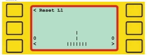
With this function you may move the finishing line electronically by adjusting the loops' amperage. Do not try this if you're not sure of what you are doing!
