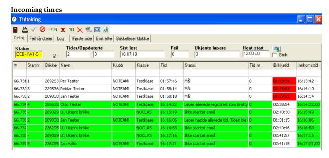
The illustration above is a typical display during timing, apart from that many common errors appear simultaneously.
