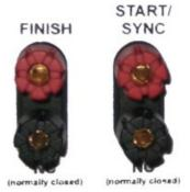
marked 'START/SYNC'. The LED marked 'Start' is red when the starting line is not in use and is green when the starting line is in use and is open (when a competitor has started.) You may also start the ETS1 by short-circuiting this contact (with a switch or a starting line) instead of pressing the 'Enter' key when adjusting the time. This may be useful when synchronising several ETS1s.
