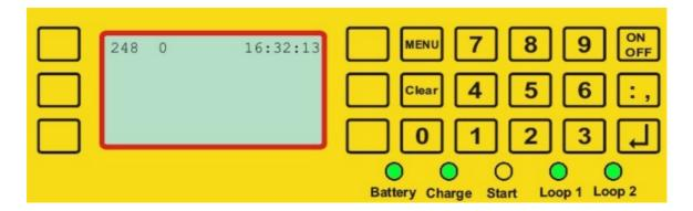
The display on the ETS1 has 7 lines and up to 20 symbols. Three keys on each side of the display control the various menu choices. In addition the keypad has numerical keys and comma, plus 4 set keys.
