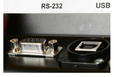
cable. The ETS1 and the PC should be switched on before connecting them to the USB cable. Connect the cable to the port marked 'USB' on the ETS1. Connect the other end of the cable to an available USB port on the PC.
