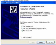
5. Select Install the software automatically (Recommended).
